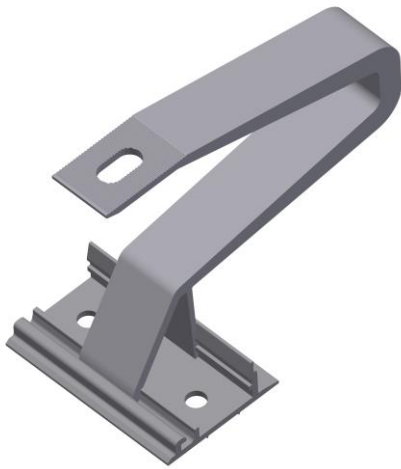
Fig. 1 Isometric view of the roof hook
