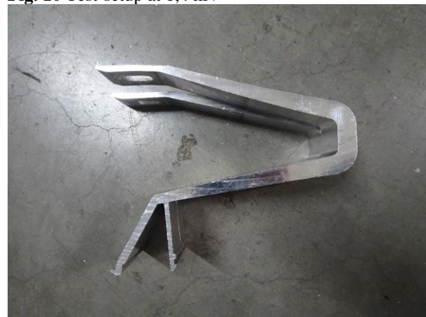
Fig. 12 plastic deformation after 45mm traverse path
