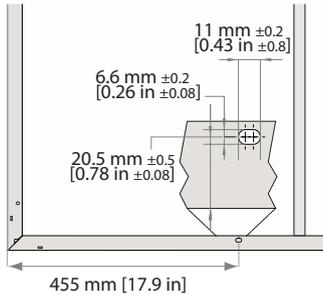
Fig. 12: Mounting holes: REC Alpha 72 Series
