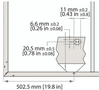
Fig. 13: Device specifications for mounting holes
