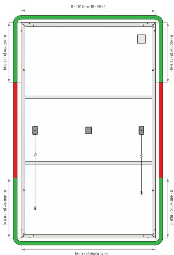
Fig. 24: REC Alpha 72 Series MLPE device installation zones
