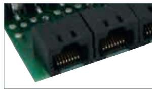
Retrofit version with RJ45 connection for existing installations.
