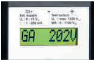
Indication of the measured sparkover voltage.
