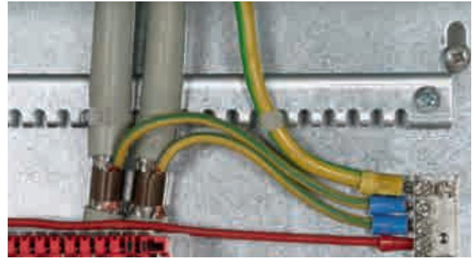
Extremely space-saving shield connection system for use as constant force spring. A spring element compensates the yield of the cable materials.
