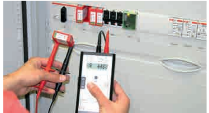
For testing the sparkover voltage of surge arresters. The specimen is connected via the included test leads or special test adapters.
