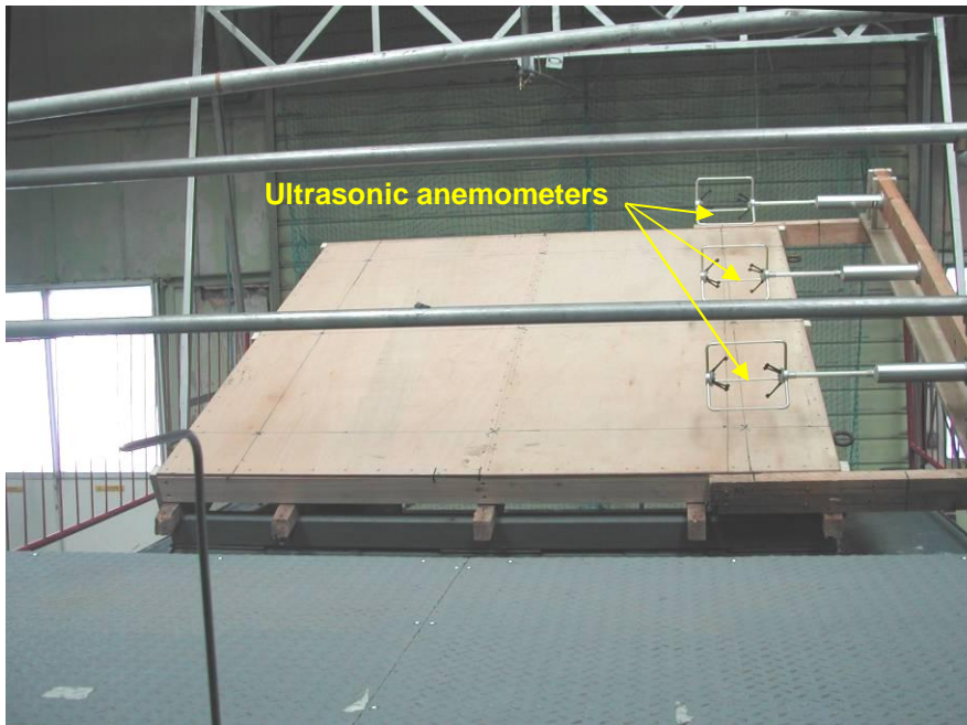
Figure A2 Calibration of the wind speed over the test specimen area
