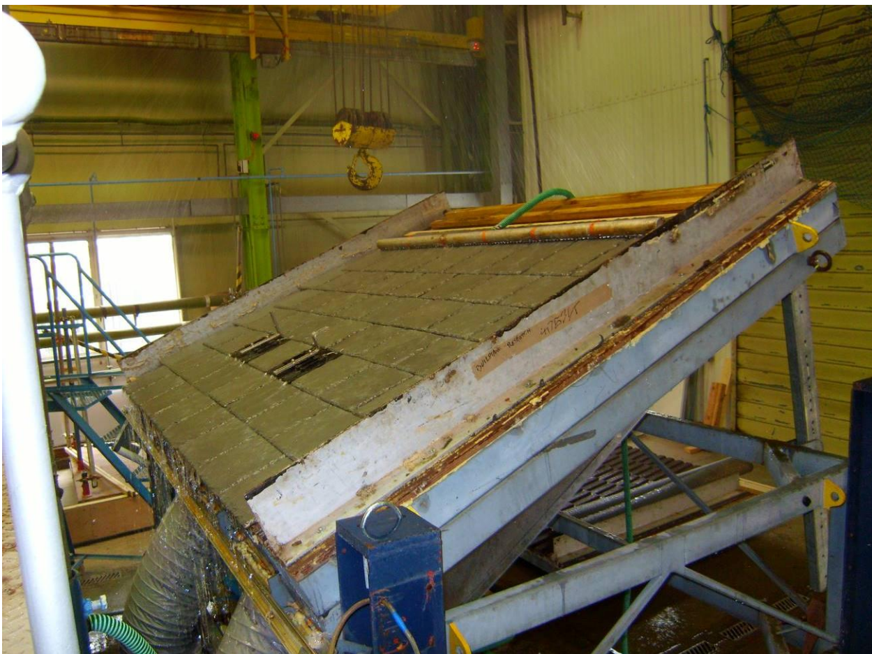
Figure 3 Solar Slate Plates under test installed with 500mm x 250mm natural slates
