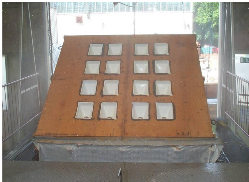
Figure A6 View of the 16 rainfall collection buckets on the test rig
