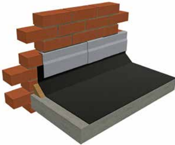
figure 04 flashing to a flat roof upstand
