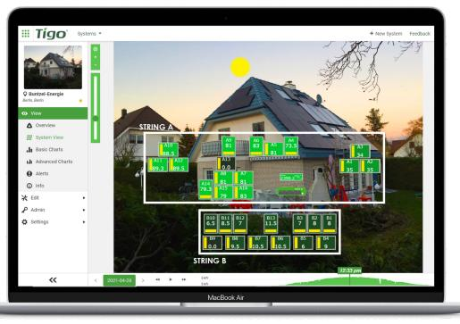
Without optimization, the inverter would choose a lower operating point for the string and the unshaded modules would contribute less than what they can produce under the site conditions. Instead, the best performing modules stay at the maximum power point set by the inverter and the optimizers adjust their output for the best result.
