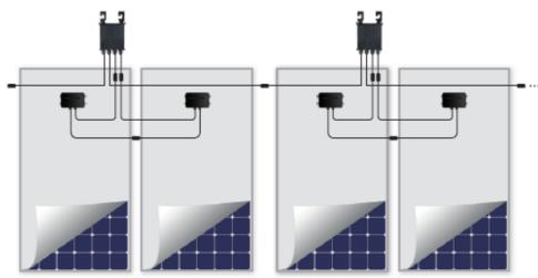
The new OP600 is a very cost effective option for commercial systems with a single power optimiser connecting to two 60 cell modules, significantly reducing the cost of the system.
