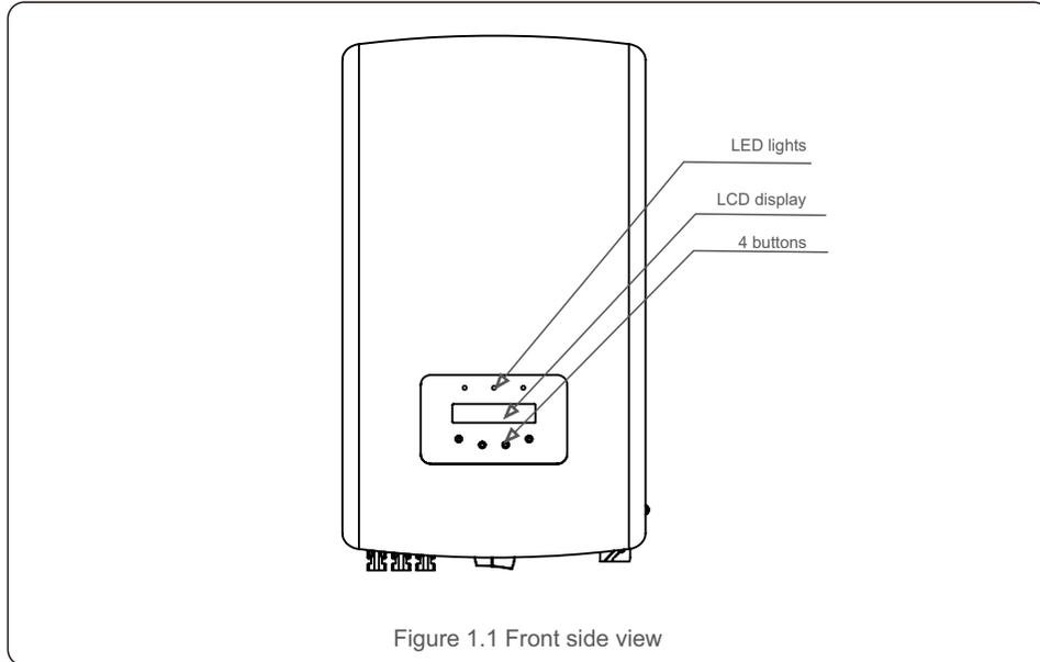
Figure 1.1 Front side view
