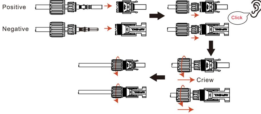
Figure 4.10 Assemble the cover of the terminal connector
