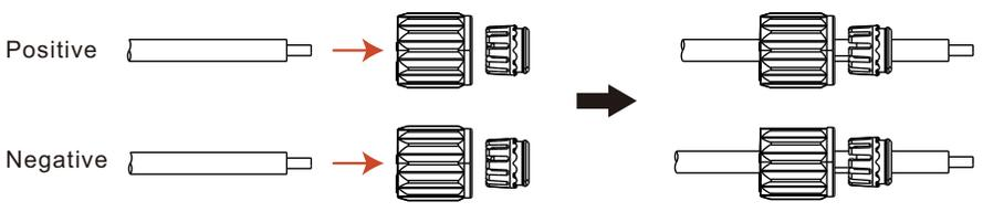
Figure 4.8 Pass the cable trough
