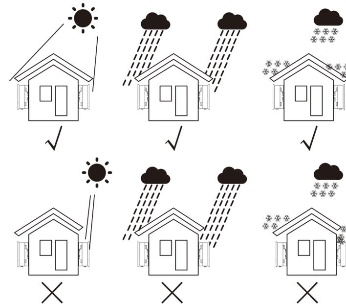
Figure 4.1 Recommended Installation locations
