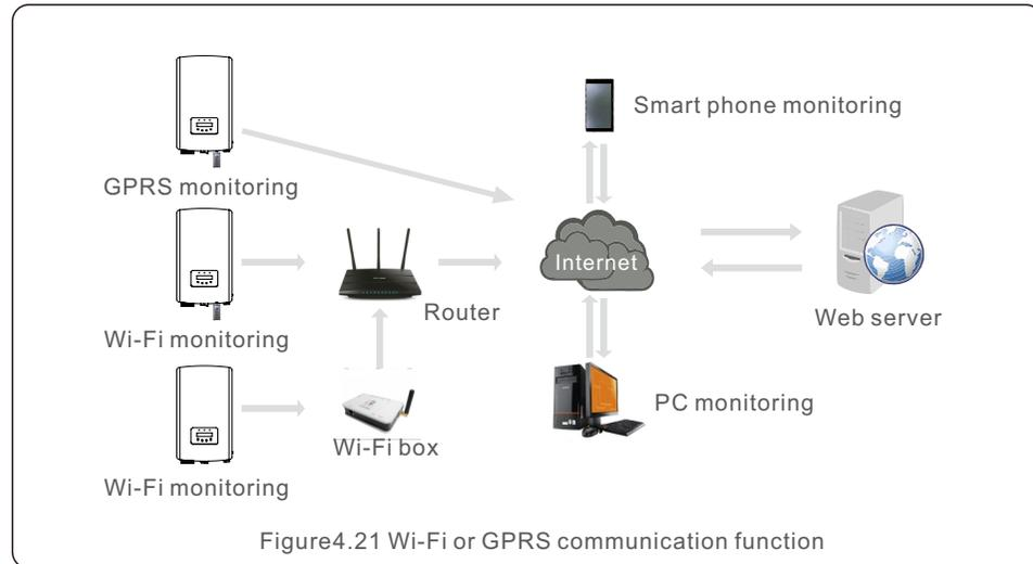
Figure 4.21 Wi-Fi or GPRS communication function
