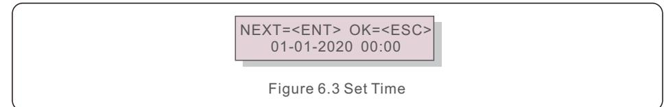
Press the UP/DOWN keys to set time and data. Press the ENTER key to move from one digit to the next (from left to right). Press the ESC key to save the settings and return to the previous menu.
