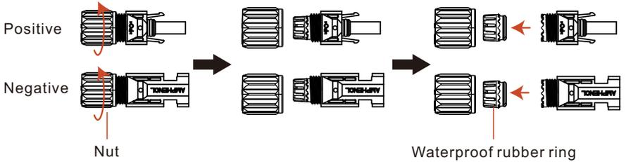
Figure 4.7 Remove the cover of the terminal connector
