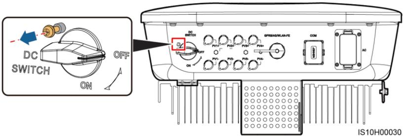
3. If there is a DC switch between the PV string and the inverter, turn on the DC switch.
