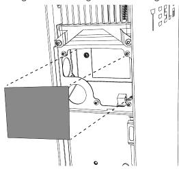
3. Attach the included drill guide to the front of the first Powerwall by bracing the inside half of the guide against the bottom of its wiring compartment.
