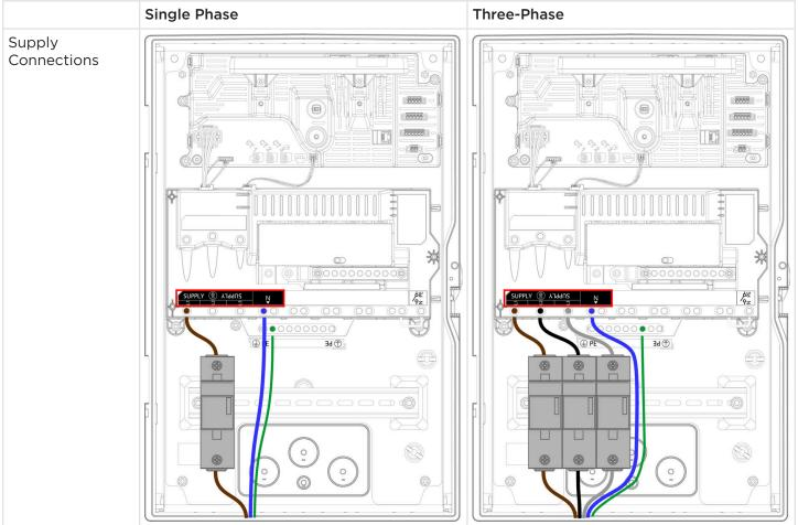
Table 2. Conductor Connections for Single Phase (left) and Three-Phase (right)
