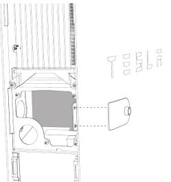
5. While holding the drill guide to make sure it conforms to the edge of the Powerwall chassis, drill a 6 mm (1/4-inch) pilot hole using the small hole in the drill guide.
