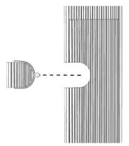
b. For back cable entry installations, remove the plug from the back cable entry port and place it in the side cable entry port.
