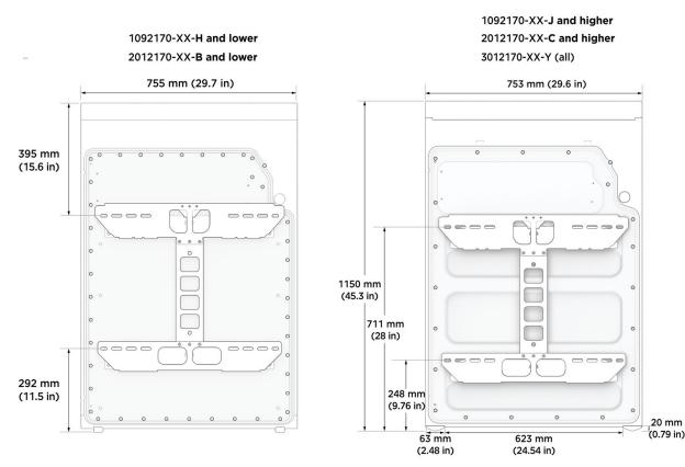
Figure 2. Powerwall 2 Identification by Mounting Bracket Height
