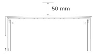
**NOTE:** The enclosure must be installed in the orientation shown below. Do not mount the Backup Gateway enclosure horizontally or upside down.
