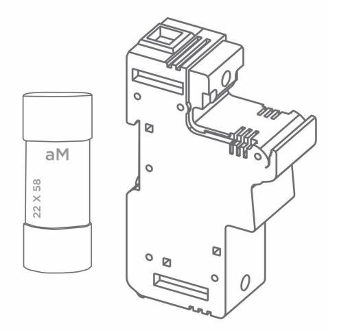
**NOTE:** The 'type aM' fuse ensures 16 kA short circuit current protection per DNO requirements. Without this fuse, the Gateway is rated to a 10 kA short circuit current. If replacing fuses or breakers, they must be of equivalent trip/open and short circuit ratings and CE marked.
