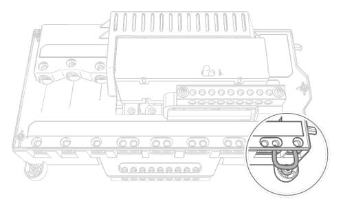
**WARNING:** To ensure safe operation, **a local earth connection must be present** on the site such as by earth rod or ground electrode. During a grid fault it cannot be assumed that the DNO's Earth or PEN conductors are intact. Installation of earth rod must comply with local codes.
