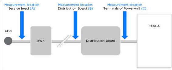
**NOTE:** The difference between the impedance point C and point A is within 0.1 ohm in a standard electrical installation.
