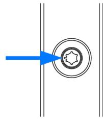
**NOTE:** The top cam is symmetrical and can be rotated in either direction to secure the side clip. The bottom cam must be rotated toward the first Powerwall so that its stepped side (indicated by the notch on the hex camshaft head) engages the housing of one of the Powerwalls.
