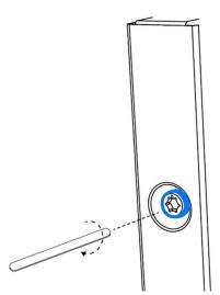
6. Place a magnetic camshaft cap on each of the four hex camshaft heads
