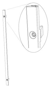
4. Slide the side clip into the gap between the two Powerwalls so that its flanges engage the side hem of each enclosure.
