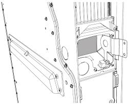
4. Clip the outside half of the drill guide to the inside half so that the guide engages the hem of the Powerwall enclosure.
