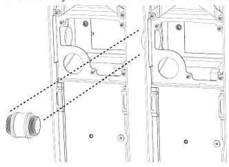
• Thread an insulation bushing onto each end of the conduit nipple, but do not fully tighten the bushings.
