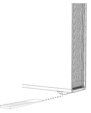
NOTE: When joined, the units should be level within +/- 2 degrees side-to-side and within +/- 5 degrees front-to-back.
