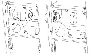
3. (All installations) Locate a side clip, making sure the flange (with magnet) is positioned at the top and that the cams are rotated vertically in relation to the clip.
