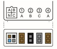
Figure 24. Neurio W2 Meter Voltage Tap Port (left) and CT Ports (right)
