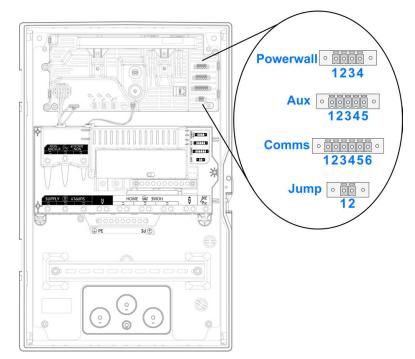
Table 6. Powerwall Communication Wiring
