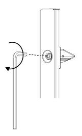
• Turn the bottom cam toward the wall (toward the first Powerwall) so that the cam indicator notch on the hex camshaft head points toward the wall, until the cam clicks into place.
