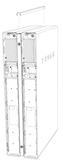
9. (Concealed wiring installations only) Tighten the insulation bushing on each side of the conduit nipple to secure the bridge between the two Powerwall wiring compartments.
