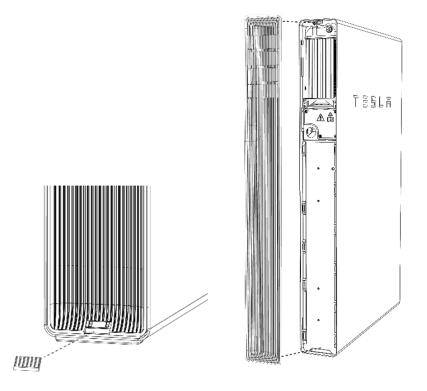
5. Using a T20 Torx bit, remove the wiring compartment covers from the previously installed Powerwall.
