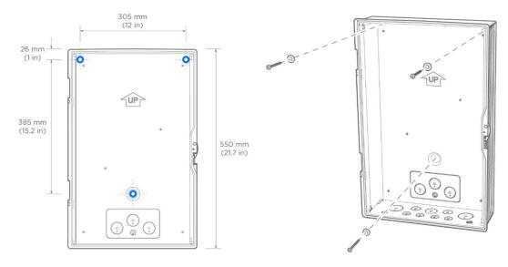
CAUTION: The sealing washers must be installed to guarantee IP55 ingress rating.
