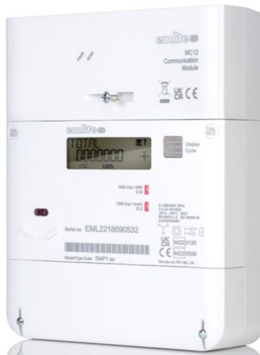
The EMP1.\* is a whole current and LV/CT 3 phase 4 wire AMR meter. Supplied inclusive with one of the latest LTE-M communications modules making it an ideal solution for most three phase installations up to 100KW. As well as MiD/MiR and IEC compliance the EMP1 range is also approved for BSC601 code of practice 5 and 10 settlement when data is collected via an approved data collector.
