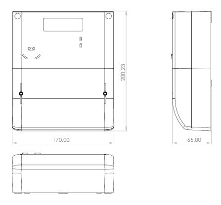
Fig. 9 - EMP1.az and EMP1.av dimensions when fitted with extended terminal cover
