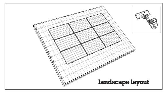
ClickFit Evo mounting system with trusshook for solar panels, for pitched roofs with roof tiles
