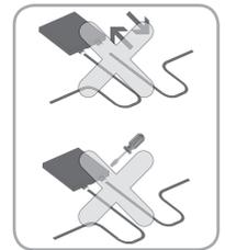
Do not bending junction box's cable. While under stress, it may occur module damage. Cable bending radius should be more than 4 times the cable diameter, at least.
