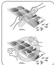
Do not approach the damaged or broken module unless you are an authorized or qualified expert. Failure to comply may result in serious bodily injury or death.
