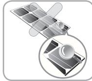
Do not apply a shock to the junction box of the module or pull the cable. Do not remove the labels attached to the module. Failure to comply may result in damage of the product.
