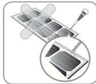
Do not artificially concentrate sunlight on the solar module surface. Failure to comply may result in product damage or failure.
