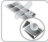
Do not apply a shock to the junction box of the module or pull the cable. Do not remove the labels attached to the module.
