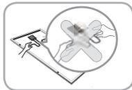
If the installing modules on curved surface, (e. g. arch type), as shown in the below picture, do not forcefully modify the module in the installation when connecting it with the structure. Only install the module in the place where the structure for the panels has been properly set up. An improper structure may cause deformation of the panels. Panels may also be damaged by unapproved installation methods such as the use of a crane.
