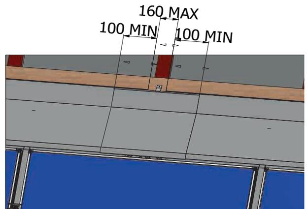
In the same way, place the corner flashings, having applied beforehand a PU glue joint on the overlapping zone of the top flashing. (Overlapping at least 100mm)
