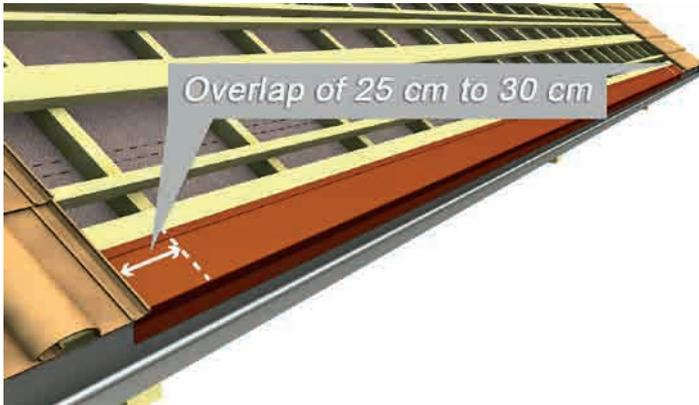
At any rate, the length and the width of the strip should be enough so that the following overlap dimensions are adhered to:
