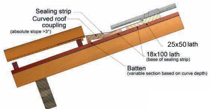
A batten is placed to fit with the thickness of the roof tile and to provide a flat base for the sealing strip.
