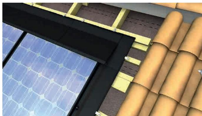
Place the precompressed seal on the flashings around the area on the lateral and upper parts.
