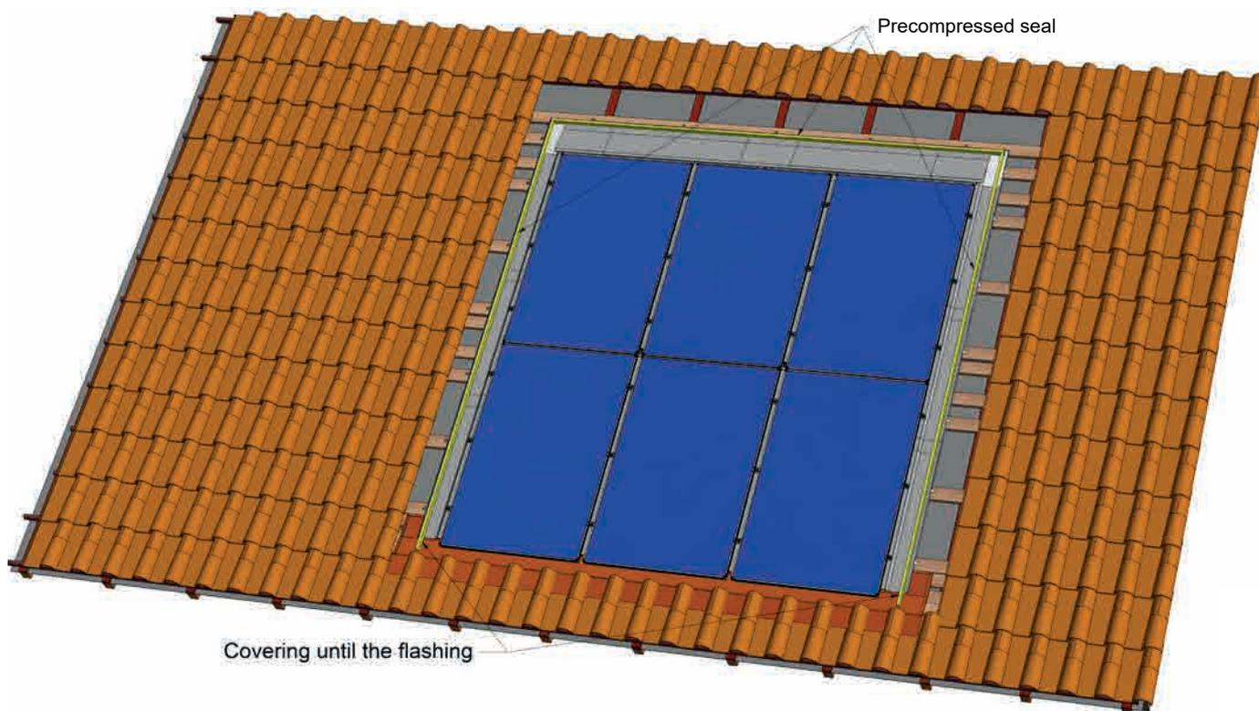
The seal must reach the bottom of the flexible flashing strip to prevent any potential infiltration of water or solid particles.
