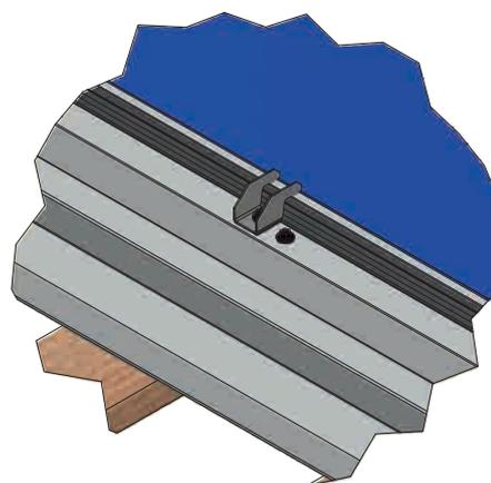
4• Place the module and attach the new assemblies (fixing clamp + EPDM foam + GSE screw).
