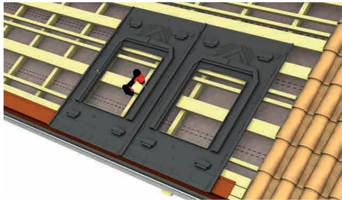
**ATTENTION: WHEN INSTALLING THE SUBSEQUENT ROWS, ADJUST HOW ONE ROW COVERS THE OTHER USING THE SCALE BASED ON THE LENGTH OF THE MODULE (CF DEVICE).**
