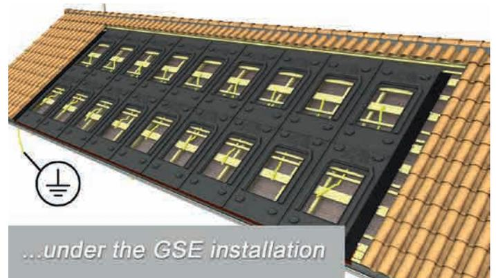
**ATTENTION:** WHEN SETTING UP THE CABLES, MAKE SURE YOU DO NOT CREATE ANY INDUCTION LOOP, IN ACCORDANCE WITH REGULATION.
