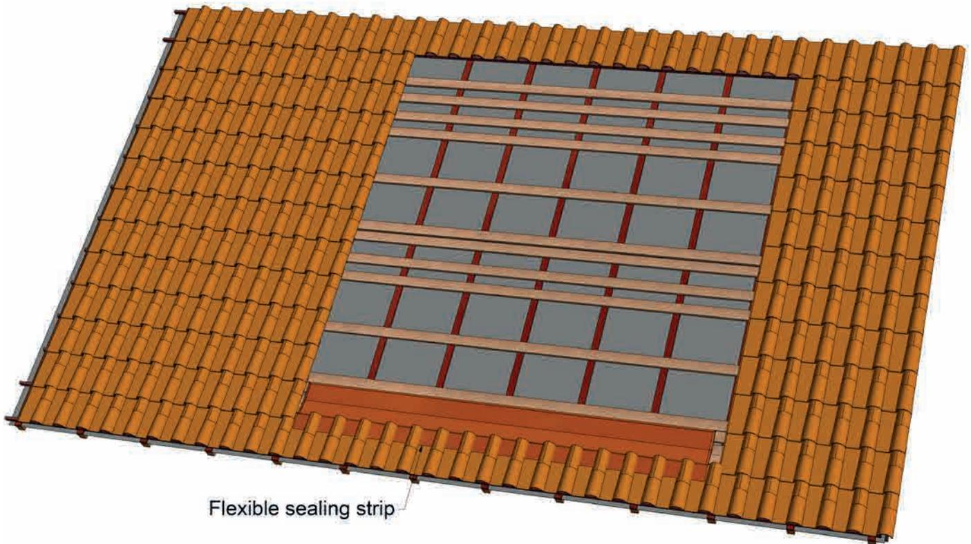
The sealing strip is laid out to link up with the bottom part of the roofing (PV array in the middle of the roofing).
