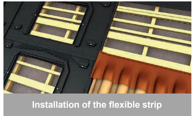
Then, position the GSE panel so that it's overlapping with the flashing strip.
