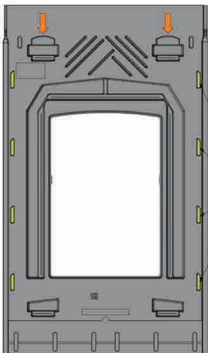
Position the modules in such a way that they're resting on the support pads (yellow) and abut against the upper pads (orange arrows).
