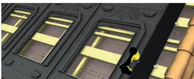
Pre-drilling of GSE frames + flashings + edge wedges
