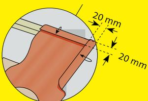
When installing the sealing strip on tiles with relief, make sure to press it down well so that it follows the roof tile's shape correctly. Make a 20-mm fold on the top part and sides to prevent water upwelling.
