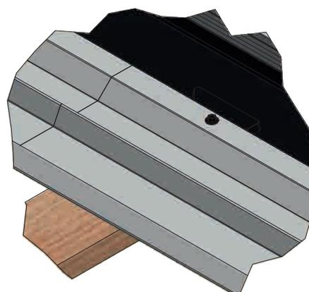
2• Screw one GSE screw at the location of old hole, having placed beforehand a new polypropylene edge wedges under the corrugation if it is located on an array edge.
