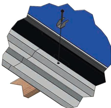
1• Unscrew the fixing clamp, remove the module and remove the edge wedges.
