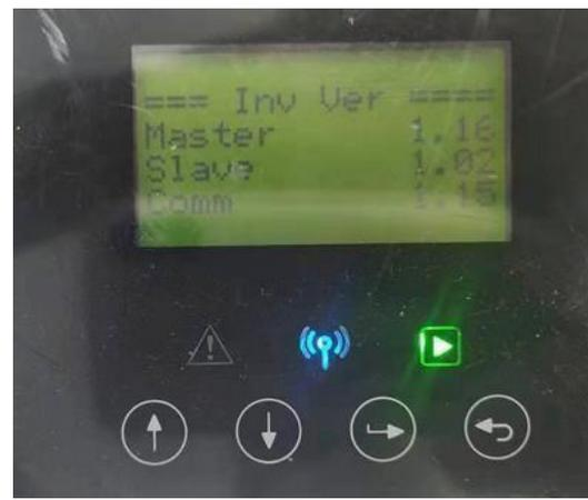
9. Turn on AC & DC breaker. If you updated the HMI, long press the “enter” and click “set” to turn on the inverter. Make sure the inverter can enter **Normal State**.
