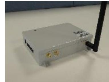
The dimensions of the EMS are W165mm x L115mm x D43mm.
