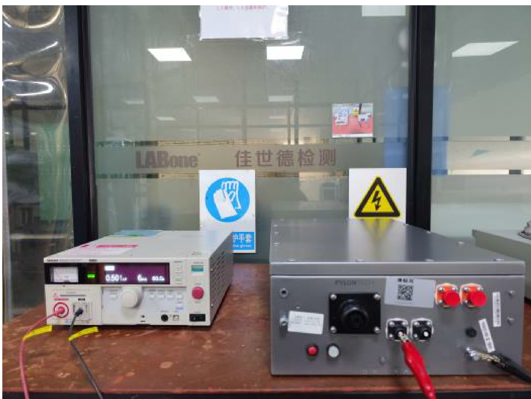
Fig.R03.6 After the test Leakage current is 6 \mu A.
