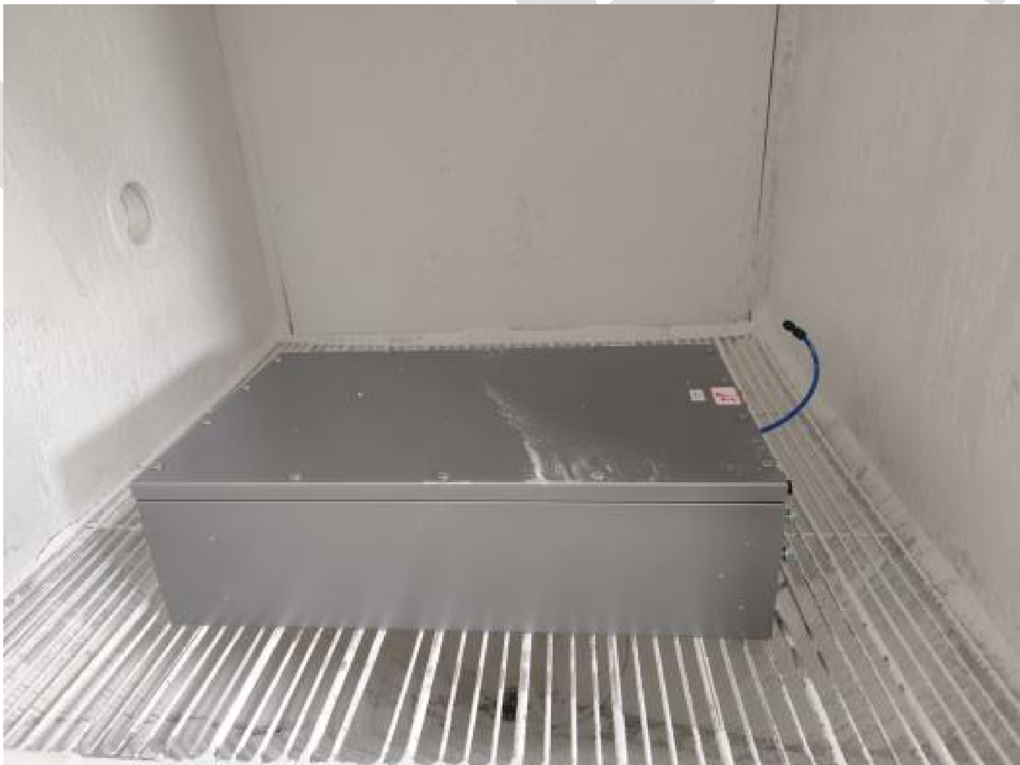
Fig.R01.3 During the test before falling dust
