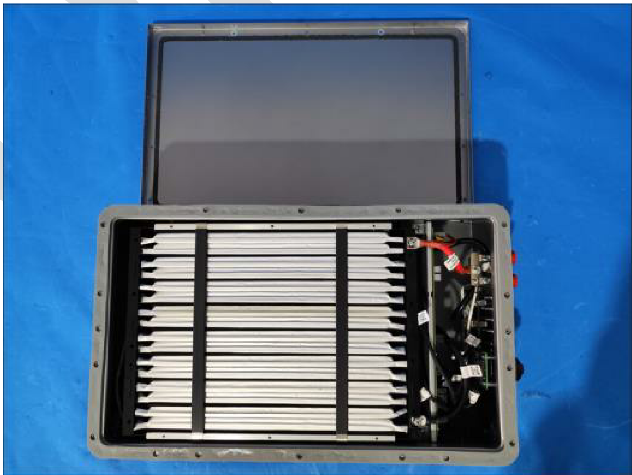
Fig.R02.4 After the test no water inside
