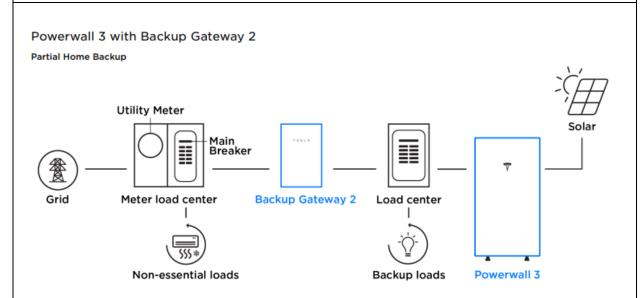
CLS is composed of Powerwall 3 and Backup Gateway 2 that controls the export on the Point of Coupling. Within the Backup Gateway enclosure is a microprocessor controlled power contactor, inclusive of line- and load-side voltage sensing and current measurement. In addition, the Backup Gateway contains a meter in which the CTs that measure the site net load connect to.
