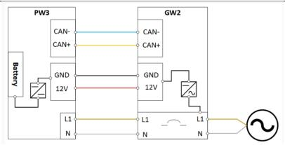
The elements considered are represented in the diagram. As can be seen, the supply of the Backup Gateway 2 (GW2) is provided by 2 paths, from Grid, and also from Battery of Powerwall 3 (PW3), that's why failure of supply has not been considered.
