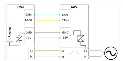
The elements considered are represented in the diagram. As can be seen, the supply of the Backup Gateway 2 (GW2) is provided by 2 paths, from Grid, and also from Battery of Powerwall 3 (PW3), that's why failure of supply has not been considered.
