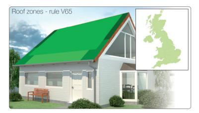
When using the new reinforced 2014 clamps, the available area to install a GSE integration roof system in wind zone 3, at 15 m in height is equal to the entire available roof area.
