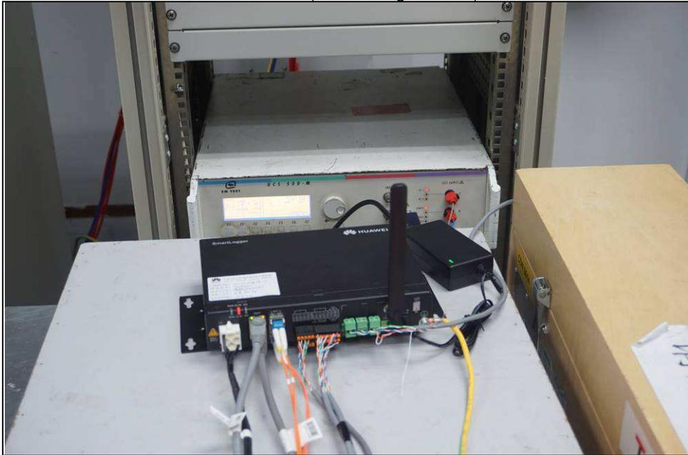
EFT TEST (12V Output Signal Line)
