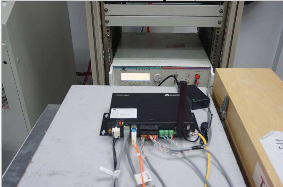
EFT TEST (DI Signal Line)
