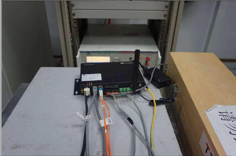
EFT TEST (GE Signal Line)
