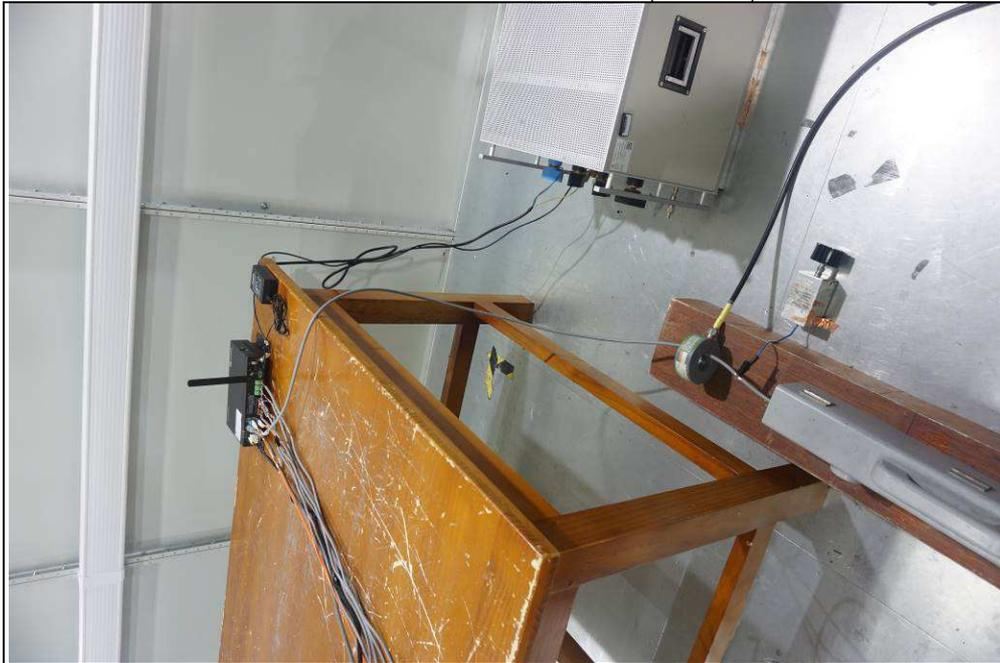
RADIATED EMISSION TEST (30~1000MHz)
