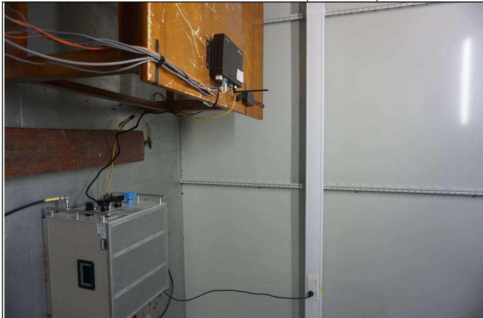
**CONDUCTED EMISSION TEST (Telecom port-RS485)**
