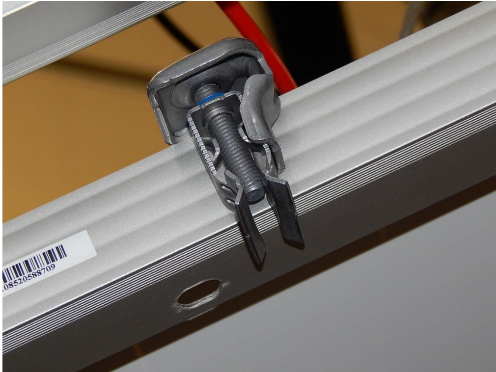
Figure 14. Image to show the RH1 roof hook under test.
