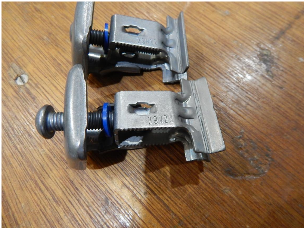
Figure 15. Image to show the RH1 roof hook under test.
