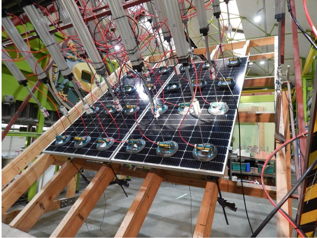
Figure 13. Image to show the RH1 roof hooks under test.
