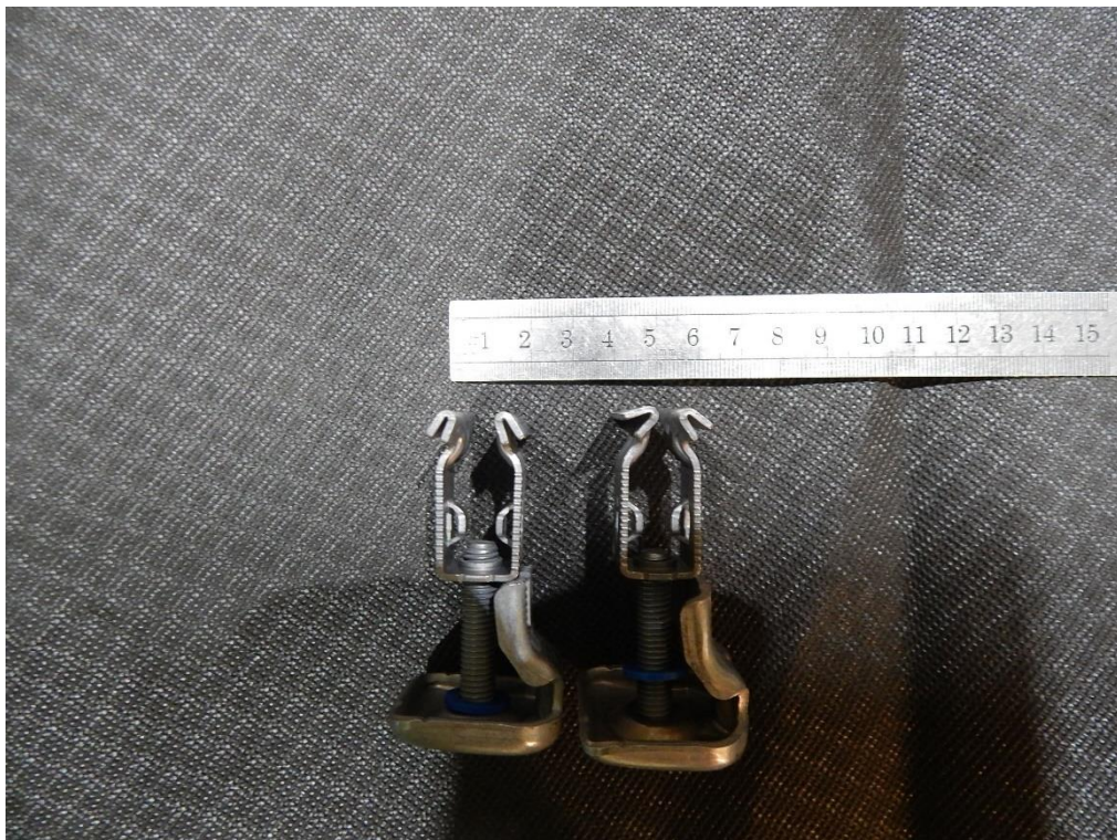
Figure 17. Image to compare the damaged clamp, right, and new clamp, left, after the buckling of the PV panel.
