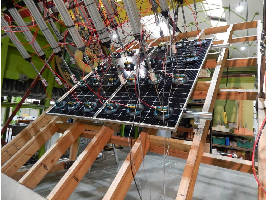
Figure 19. Image to show the hanger bolt system under test.
