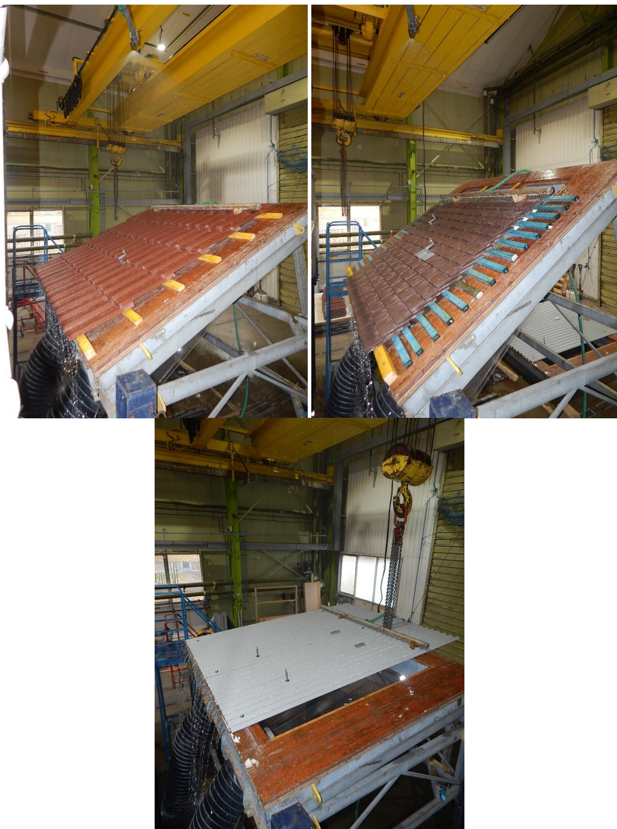
Figure 11. The test specimens under deluge test (RH1 roof hook top left image, RH Flat roof hook top right image, Metasole Bracket and Hanger Bolt bottom centre image).
