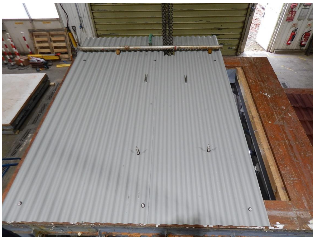
Figure 8. Hanger bolt and Metasole bracket installed on the BRE test rig prior to test.
