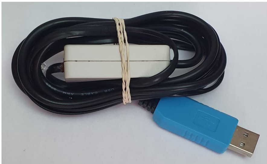
Figure 1: Pylontech US3000C cable for monitoring module
