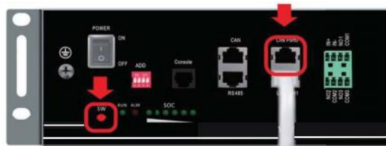
Figure 3: The master battery is defined as the battery with Link Port 0 OPEN as per the picture above.
