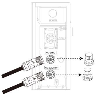
10. Connect the AC grid cable to the main panel, and the AC backup cable to the subpanel. Figure: Connect to the grid and backup loads.
