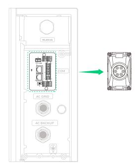
2. Rotate to remove the locking cap from the wiring compartment cover and take out a waterproof plug. Figure: Take out a waterproof plug.
