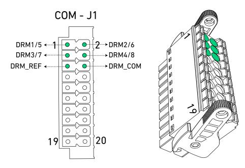
Refer to the appropriate wiring diagram and switch table to help connect.
