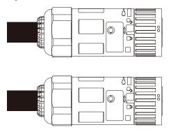
9. Remove the dustproof covers from the AC power ports. Then, insert the AC grid connector (female) to the AC grid port, and insert the AC backup connector (male) to the AC backup port. Rotate the locker in the locking direction to tighten the connectors.
