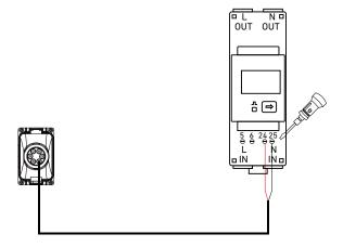
8. Connect power wires to the grid-side power sensor.
