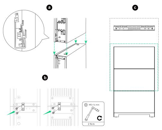
Figure: Mount the power module.
