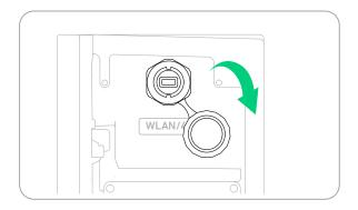
③ Install the appropriate dongle according to the networking methods.
