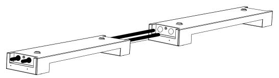
• For wall mounting, route cables into the second column from the back of the first column. Figure: Conduit run for wall mounting.
