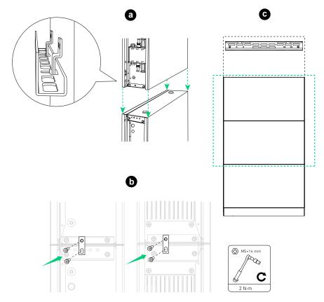
Figure: Mount the power module.
