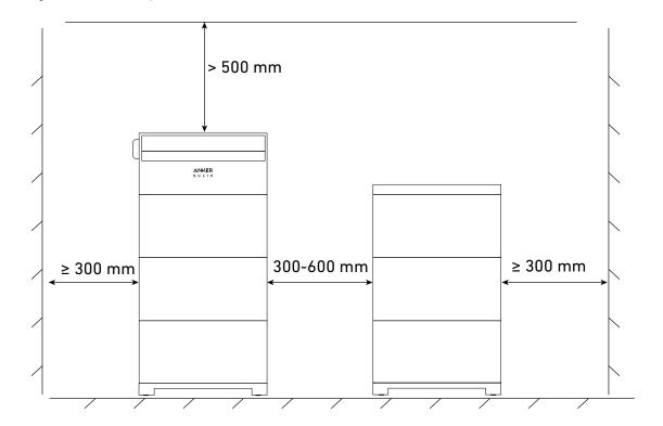
Figure: Installation space for wall-mounted modules.
