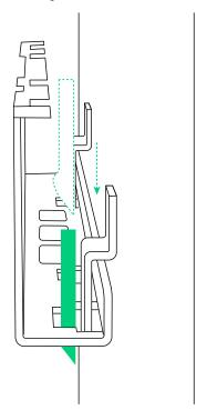
3. When adding the second column, attach the top cover to the top battery module using the screws (M5×14 mm, included). Figure: Install the top cover for the second column.
