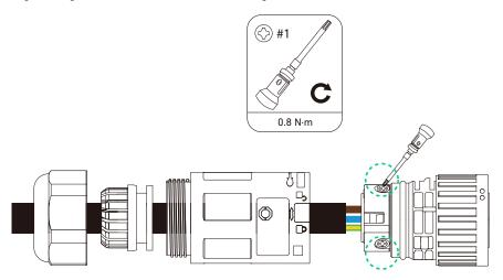
6. Align the locker and the body, and rotate the locker until you hear a click. Figure: Reassemble the AC grid connector.
