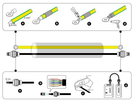
③ Install the GND cable and RJ45 signal cable.
