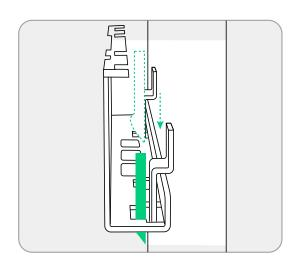
3. When adding the second column, attach the top cover to the top battery module using the screws (M5×14 mm, included). Figure: Install the top cover for the second column.
