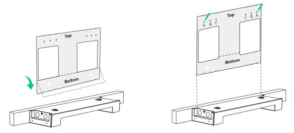
2. Repeat the previous step to mark any remaining pilot holes as necessary. Figure: Mark pilot holes for remaining modules.
