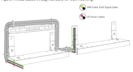
② Assemble the GND cable and RJ45 signal cable.
