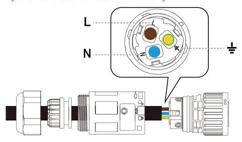
5. Tighten the three screws on the housing with a No. 1 Phillips screwdriver.
